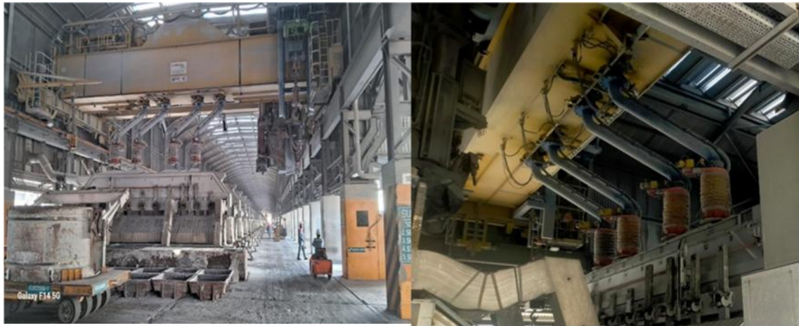
Figure 1. Left: crane usage to feed alumina to pots; Right: crane usage to feed alumina to pots.
